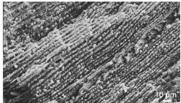
**Fig. 13.** SEM image of a transverse fracture surface of a rat long bone showing a vast area of aligned lamellae.
